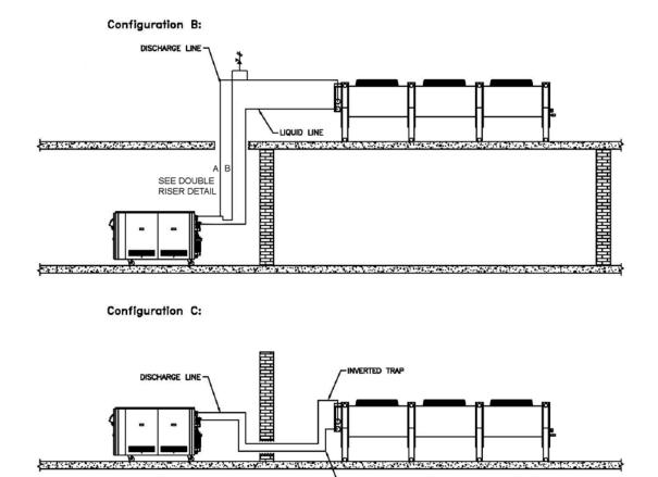
Figure 8: Remote Condenser Configurations
